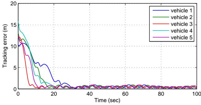
Fig. 7. The tracking error of each vehicle  $i$ ,  $\|q_i - q_0\|$ , with smaller  $r_i$ .
