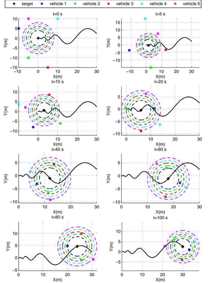
Fig. 4. The positions of each vehicle  $i$ ,  $p_i$ ,  $i = 1, \dots, N$ , at some instants.
