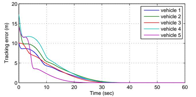
Fig. 10. The tracking error of each vehicle  $i$ ,  $\|q_i - q_0\|$ ,  $i = 1, \dots, N$ .
