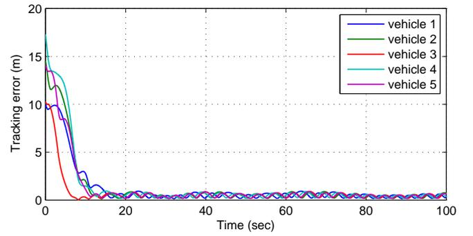
Fig. 8. The tracking error of each vehicle  $i$ ,  $\|q_i - q_0\|$ , with larger  $v_i$ .
